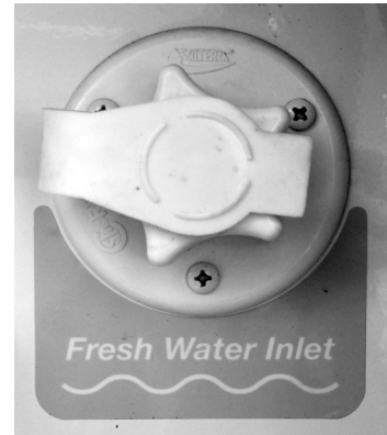
Fresh (City) Water Connection “Fresh Water Inlet” (Located in the water service center) -Typical View
