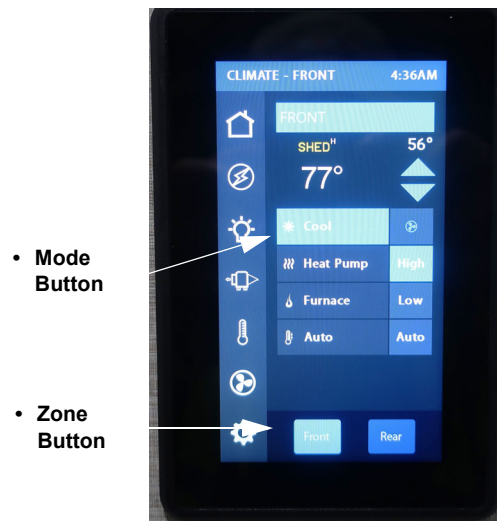
Thermostat "Climate" Screen (Located on Multiplex Monitor Panel)
