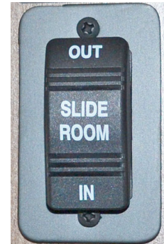
Slideout Switch -Typical View
