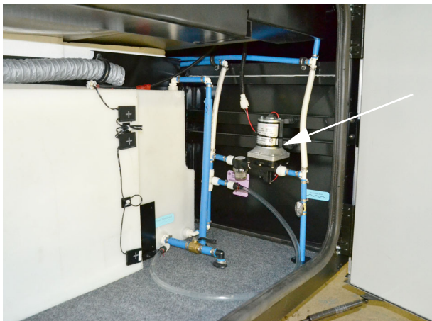
Water Pump (Located in a passenger side compartment) *Models 38F and 38W
