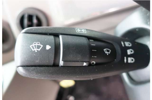
Turn Signals/High-Low Beams (Located on the left hand stalk switch on the steering column. Typical View - your motorhome may differ depending on model)
